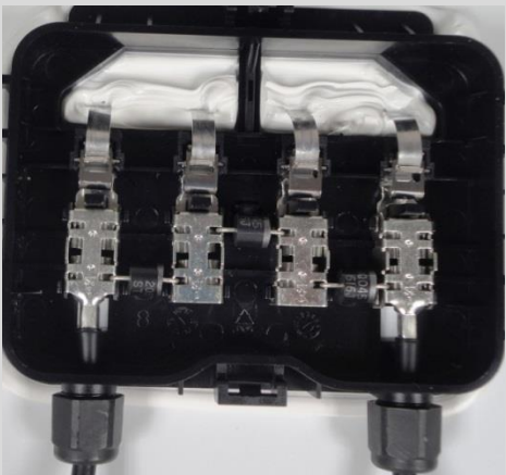
Fig.4:detail view of the Open junction Box
