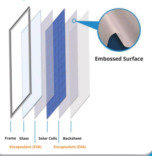
'CONSERV P 360 - 14 FC' is a wide process window curable, PID resistant, UV and weather stable Ethyl Vinyl Acetate (EVA) PV Encapsulant, proven for single stage as well as short cycle multi stage lamination processes. This Encapsulant is specially recommended for PV Crystalline Modules used in tropical (Hot and Humid) climatic conditions.
